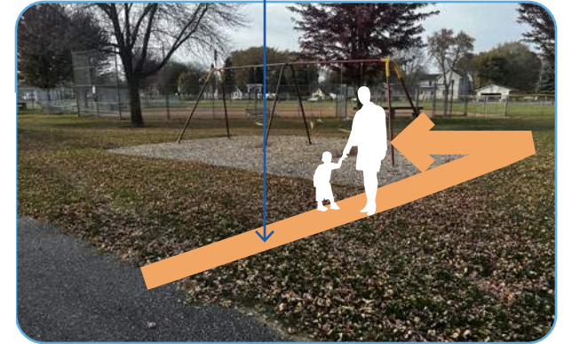
Replace the gravel path outside of the restroom facilities with an accessible concrete sidewalk
